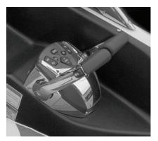
engine. In the same way, the right (or starboard) lever operates the starboard-side engine. When the two levers are in the same position, the engines work together to move the boat in a straight line. When the two levers are in different positions, the boat responds by pivoting or spinning in one direction or the other, according to the positions used.
