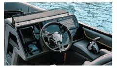
**Redesigned Captain's Helm** A new dashboard layout and design dedicates 4 unique sections of the helm to key functions, ensuring that phone charging, radio control, vessel monitoring, and vessel switching are accessible and intuitive.
